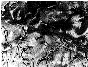
Figure: Optical microscope photograph of a thin film of freely suspended nematic liquid crystal after a temperature quench. [Credit: Chuang et al. (1991).]
